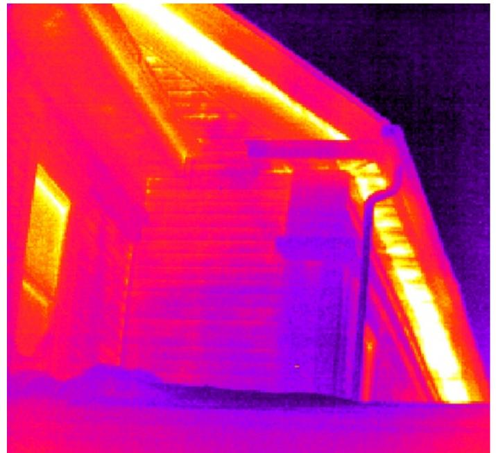
*Infrared testing can pinpoint and prioritize any facility's energy loss problems.*
