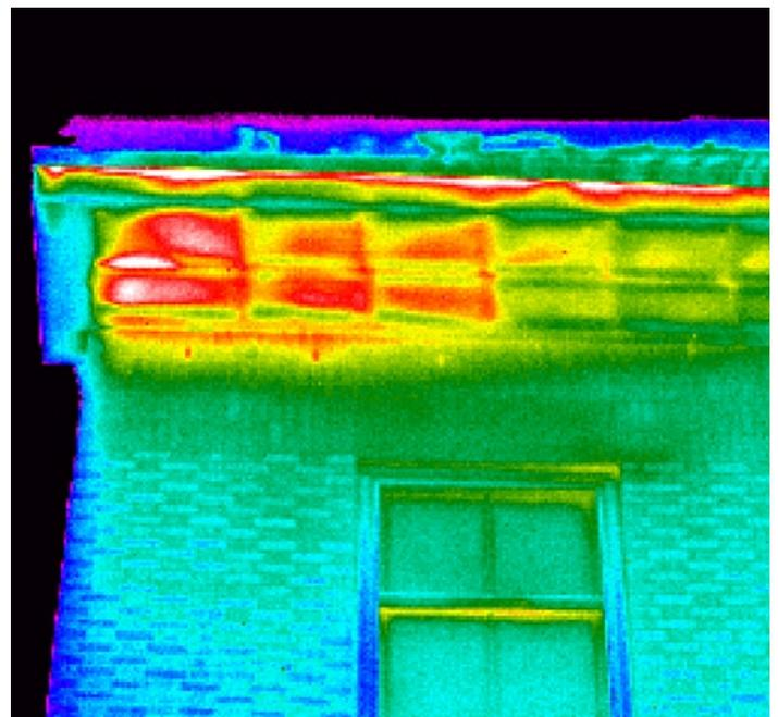
*Ice dams are often caused by excessive heat losses near the eaves.*
