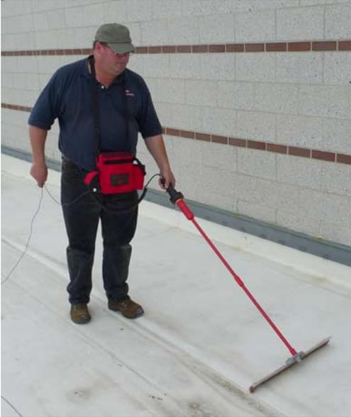
Electronic vector mapping is a cutting edge technology that is redefining the art of leak detection and quality assurance in low-slope roofing systems and many types of waterproofing applications. Vector mapping pinpoints breaches in the roof membrane by tracing the flow of an electric current across the membrane surface. Already Europe's most widely-used method for detecting roof leaks, vector mapping is rapidly being adopted by manufacturers, contractors, and specifiers in the United States.
